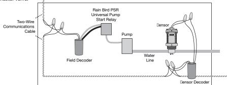
Rain Bird recommends using the FD-101 field decoder for most pump start relays and a FD-102 for larger pumps (3/4 HP and greater).
